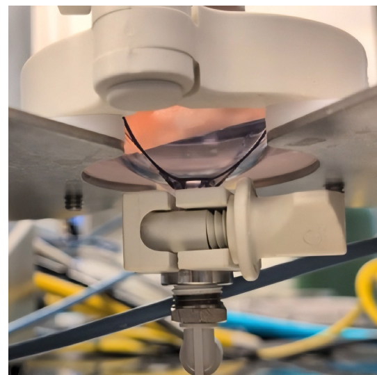
Figure 3. Photo of Pump Cycle at Halfway Point of a Liquid Out Cycle with Cell Culture Visible
